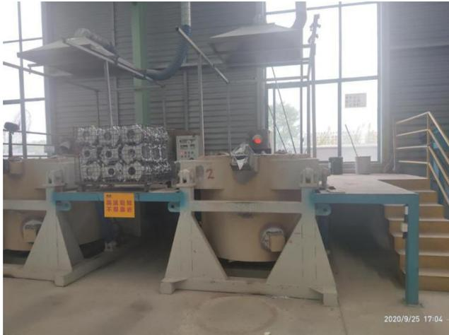
图7 熔炼炉集气罩
